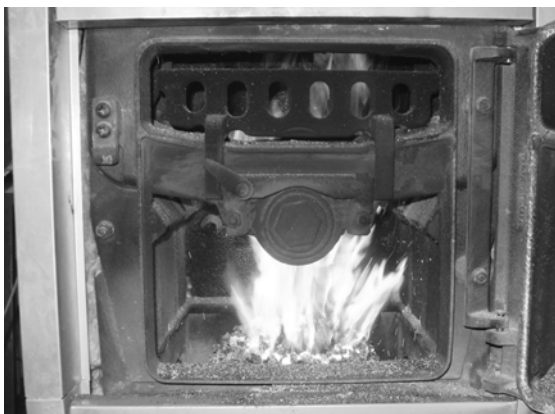
Fig.No. 27 Optimal shape of the flame
